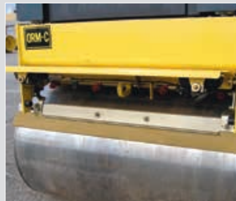
Wind protected, quick-disconnect spray nozzles with dual scrapers per drum.
