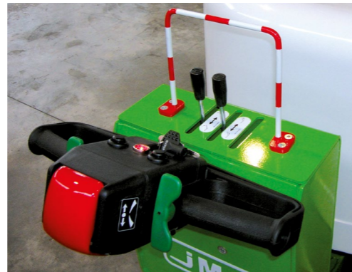
TILLER WITH BOOM AND WINCH LEVER CONTROLS
