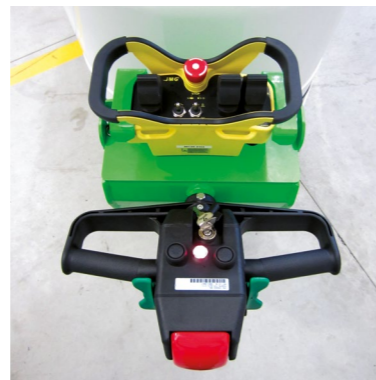
TILLER WITH RADIO REMOTE CONTROL (AS OPTION) FOR BOOM AND WINCH MOVEMENTS
